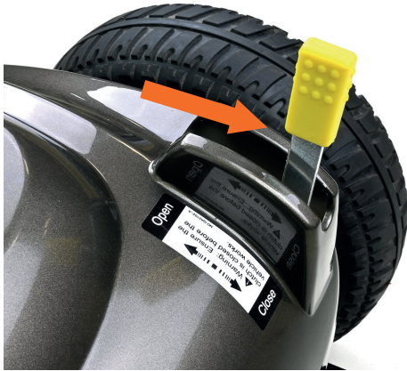
Fig 6.7.1 Drive Mode (Closed)
