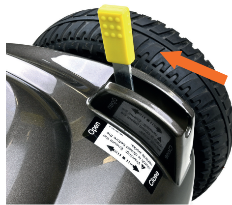
Fig 6.7.2 Freewheel Mode (Open)
